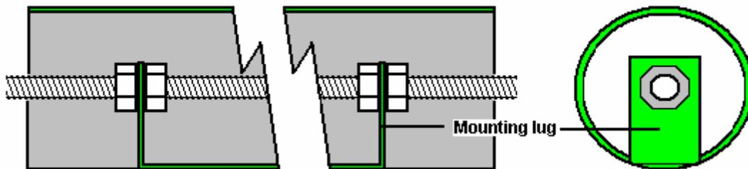
The inner nuts are manoeuvred on inside on of the lugs by hand and then the threaded rod is rotated to move one nut to the inside of the other lug, while the nearer nut is held to prevent it rotating. When the rod is positioned correctly and the inner nuts are pressed up hard against the lugs, then a box spanner is used to lock the outer nuts tightly against the lugs, forming a strong mounting lock.
