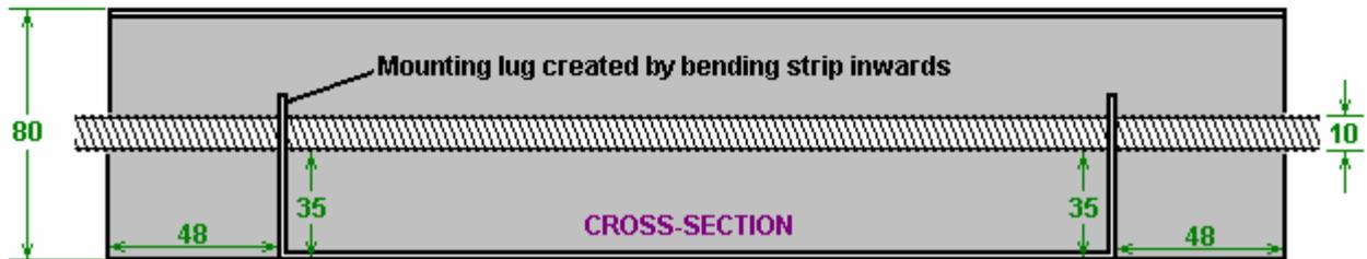
The inner cylinder is secured in position by two bolts as shown here:
