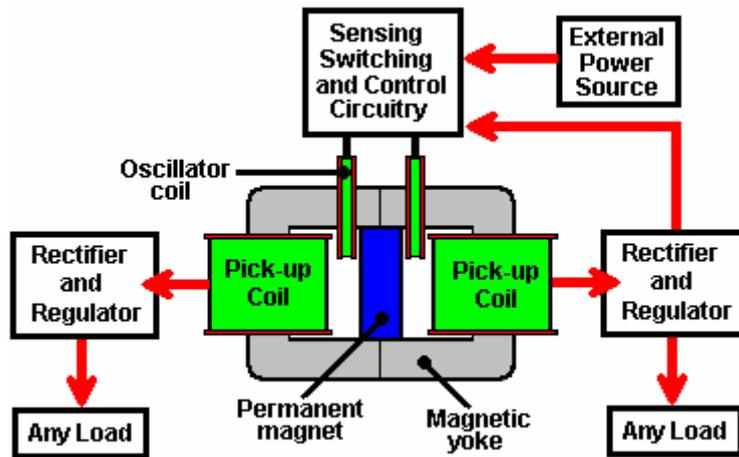
The external power source shown above is intended to be disconnected when the circuit starts operating, at which time, part of the output from one of the pick-up coils is fed back to power the circuit driving the oscillator coils. The circuit then becomes self-sustaining, with no external input but with a continuous electrical output.
