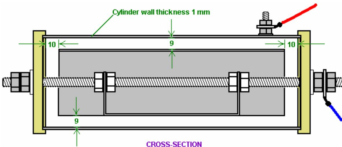
This gives a 9 mm clearance between the two cylinders and this gap stretches 360 degrees around the cylinders. The inner cylinder is located 10 mm clear of the Lexan end discs.
