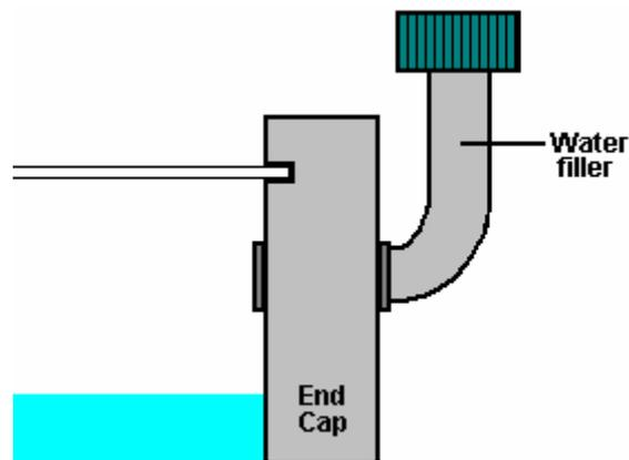
This arrangement has the advantage that it does not require a filler hole to be drilled through the steel cylinder.
