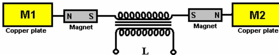
It is claimed that on switching on the primary circuit, "separation of charges" takes place with M1 becoming positively charged and M2 becoming negatively charged and that these charges are "magnetically polarised" when they formed, owing to the presence of the magnets. When the primary circuit is switched off, a "reversing current" flows in the secondary but the magnets "do not exert a polarising effect on this reversal".
