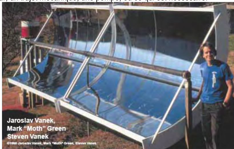
Above: Steven Vanek with his machine which uses solar thermal energy to make ice.
