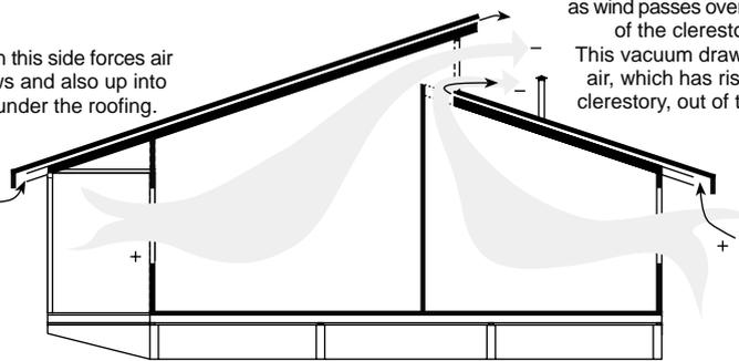
A low pressure area is developed as wind passes over the top edge of the clerestory roof.
