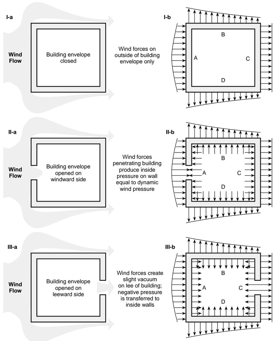
away from the wall, represent vacuum. The curved lines are a rough representation of a graph of the pressure/vacuum forces, showing how they vary in different locations.
