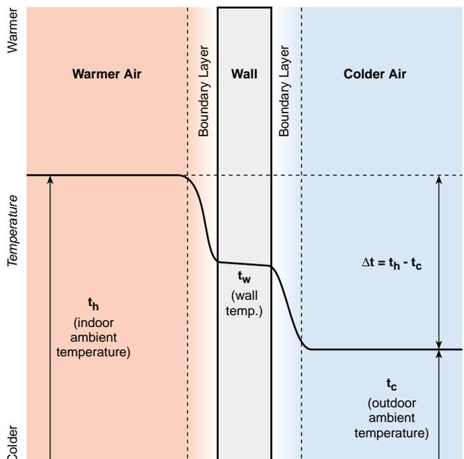
will heat up more than the air some distance away. When this situation exists, the change in temperature ( $\Delta t$ ) between the warm wall and the warm layer of air is reduced. This cuts back on heat flow.
