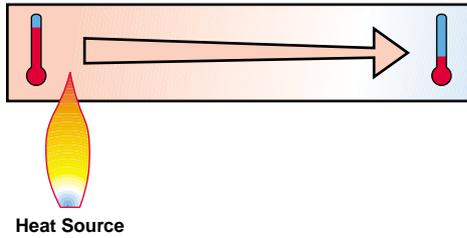
What is happening here is that the heat source is exciting the molecules in the copper to vibrate more enthusiastically, becoming more and more energetic as the temperature increases. As these copper molecules pick up physical motion from the heat energy, they continuously “bump” into the molecules next door.
