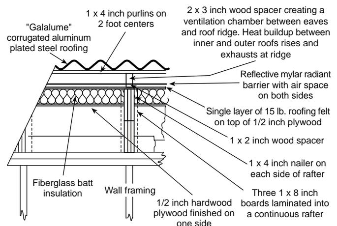
The lower sandwich contains the structure as well as fiberglass batt insulation to block conductive heat flowing downward into the living area. As mentioned in Part I, radiant heating is the principal mode of heat flow downward. Conductive heat does not move as readily downward through materials.
