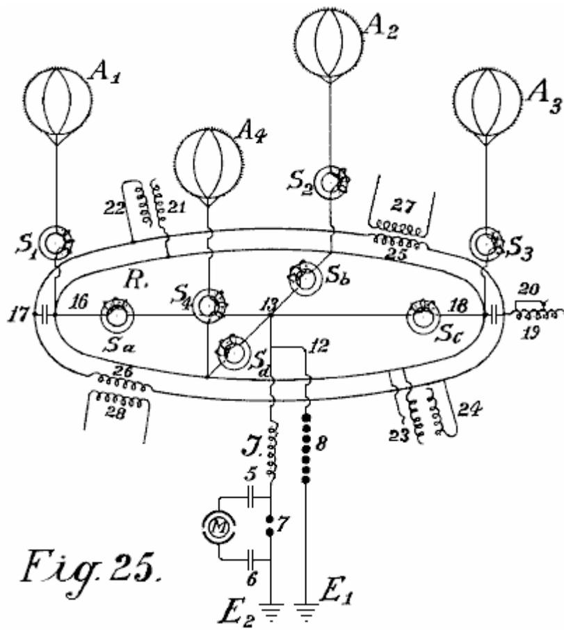
Fig.25 and Fig.26 show modified collector balloon arrangements.
