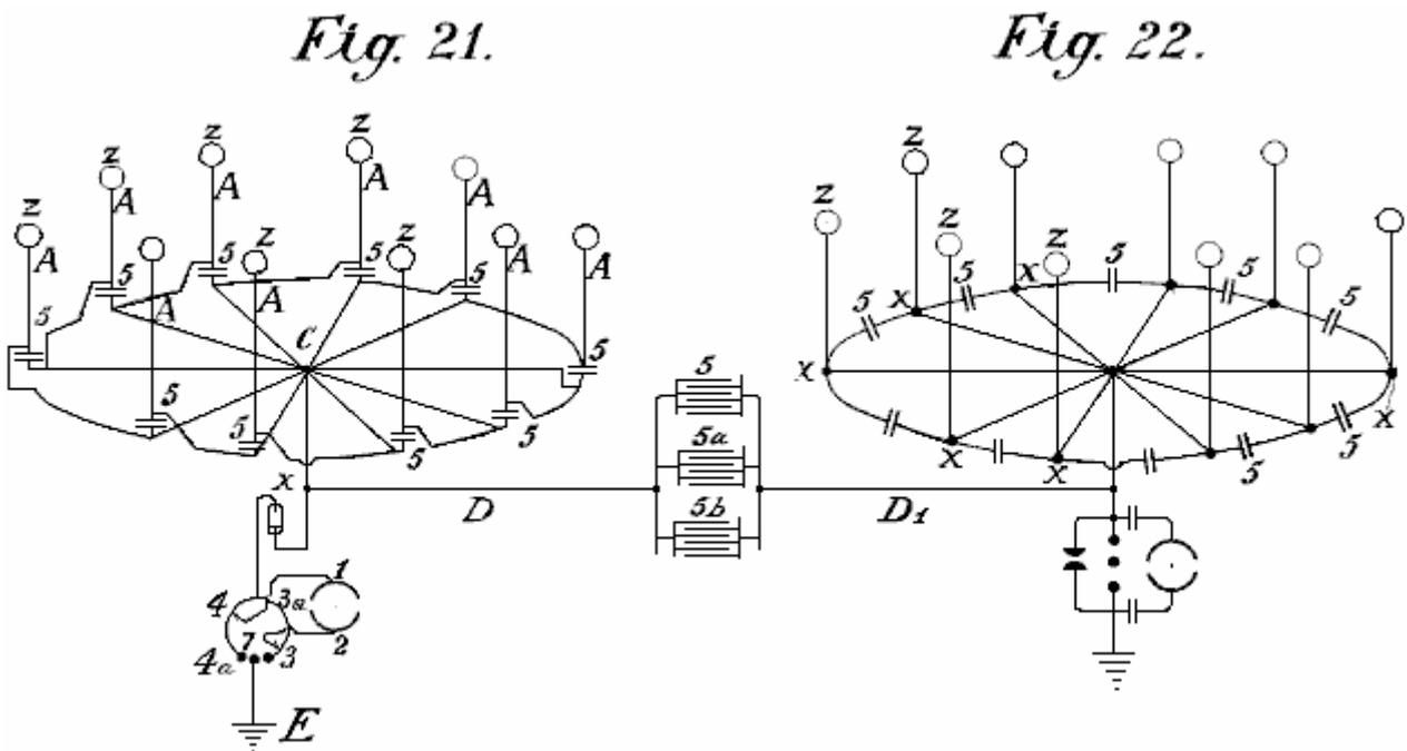
**Fig.21** shows diagrammatically, an arrangement suitable for collecting large quantities of energy.
