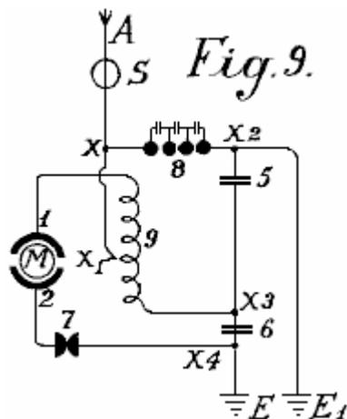
**Fig.9** shows a loosely coupled system intended for small motors for measuring purposes. **A** is the aerial, **S** is the electromagnet or aerial inductor, **9** the inductor, **7** the spark gap, **5** and **6** capacitors, **E** the earth, **M** the motor, and **1** and **2** the stator connections of the motor which is directly connected to the oscillator circuit.
