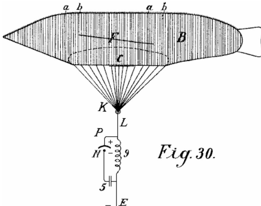
**Fig.30** only shows the difference that instead of a round balloon, a cigar-shaped one may be used, also, a capacitor **5** is inserted between the incandescent cathode and the earth conductor so that a short-circuited oscillation circuit over **P N 5**
