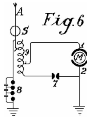
**Fig.6** shows how the oscillation circuit may have a motor connected via a variable inductor which opposes any excess voltages which might be applied to the motor. By cutting the separate coils **9** (coupled inductively to the aerial) in or out, the inductive action on the motor may be more or less increased, or variable aerial action may be exerted on the oscillation circuit.
