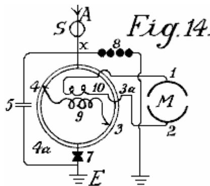
As this prevents the whole of the oscillation energy acting on the motor, it is better to adopt the modification shown in Fig. 14. The only difference here is that the motor is not wired directly to the segments of the commutator, but instead it is
