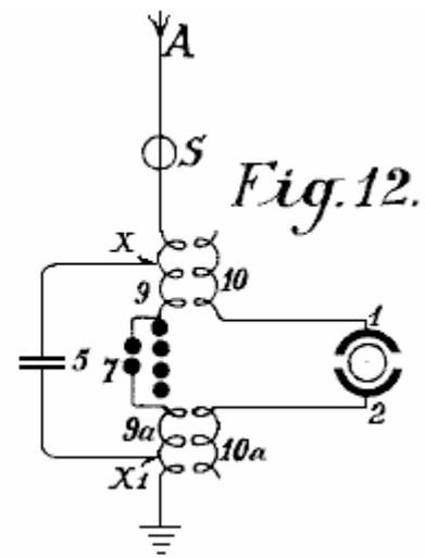
Fig. 10 shows a motor circuit with purely inductive coupling. The motor is connected with the secondary wire 10 as may be seen in Fig. 11 in a somewhat modified circuit. The same applies to the circuit of Fig. 12.
