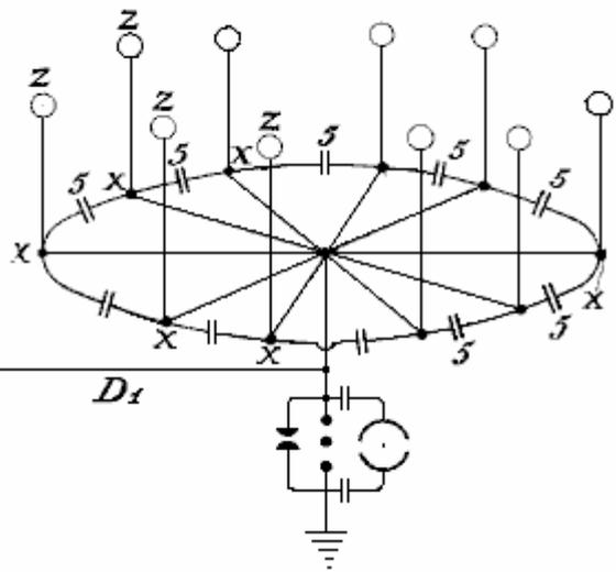
In order to collect large quantities of electricity with few aerials, it is as well to provide the aerial conductor with sets of capacitors as shown in the two methods of construction illustrated in **Fig.21** and **Fig.22**. In **Fig.21** the set of capacitors **5** is connected between the aerials **Z** via lead **A** and an annular conductor from which horizontal run to the connecting points **C** to which the earth wire is connected. **Fig.22** shows a similar arrangement.
