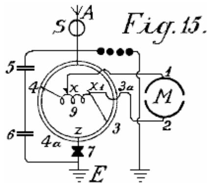
In **Fig.15**, the motor is wired directly to the primary coil at **x** and **x1** after the principle of the auto-transformer. In **Fig.16**, instead of an inductor, capacitor **6** replaces the inductance and is inserted between the segments **3a** and **4a**. This has the advantage that the segments **3a** and **4a** need not be made of solid metal, but may consist of spiral coils which allow a more exact regulation, and high inductance motors may be used.
