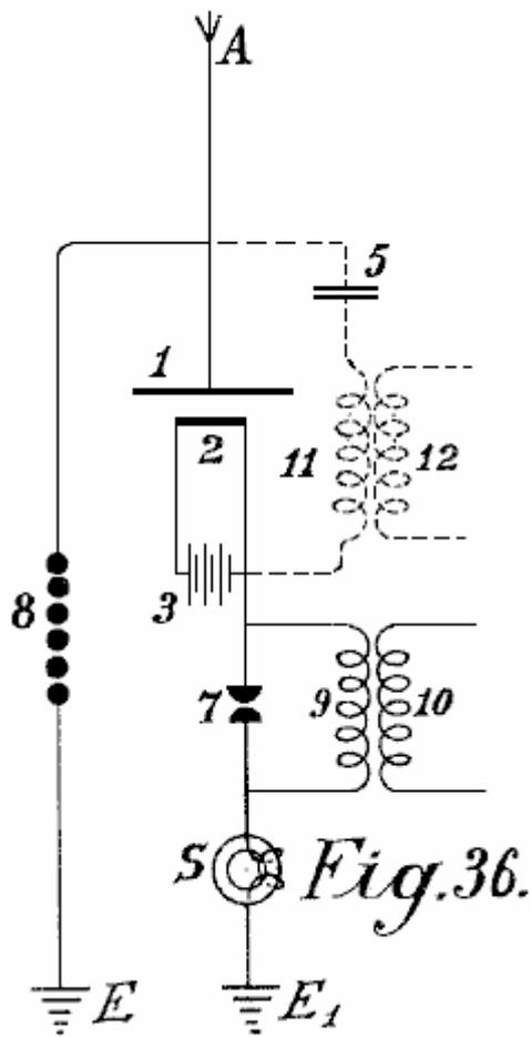
Fig.36 shows an incandescent collector with Nernst lamp
