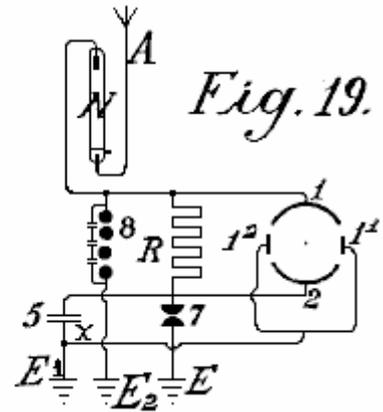
The circuits shown in **Fig.17**, **Fig.18** and **Fig.19** may be used with resonance and particularly with induction capacitor motors; between the large stator induction capacitor surfaces, small reversing pole capacitors are connected which are lead together to earth. Such reversing poles have the advantage that, with large quantities of electrical energy, the spark formation between the separate oscillation circuits ceases.
