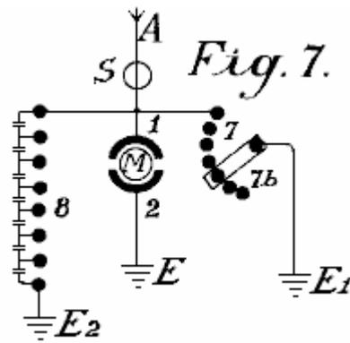
In **Fig.7** the oscillation circuit is closed through the earth (**E** and **E<sub>1</sub>**). The spark gap **7** may be increased or reduced by means of a contact arm **7b**.
