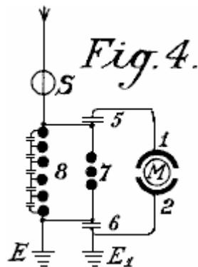
**Fig.4** is a diagram showing the protective circuitry.
