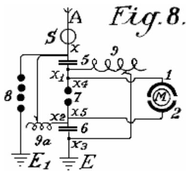
Fig. 8 shows a unipolar connection for the motor
