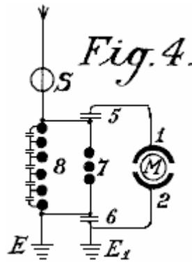
In **Fig.4**, spark gap **7** is shunted across capacitors **5** and **6** from the motor **M**. This arrangement provides improved over-voltage protection for the motor and it gives a uniform excitation through the spark gap **7**.
