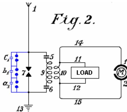
An elementary form of the invention is shown in **Fig.2** in which two spark gaps in parallel are used, one of which may be termed the working gap **7** while the second serves as a safety device for excess voltage and consists of a larger number of spark gaps than the working section, the gaps being arranged in series and which are bridged by very small capacitors  $a_1, b_1, c_1$ , which allow uniform sparking in the safety section.
