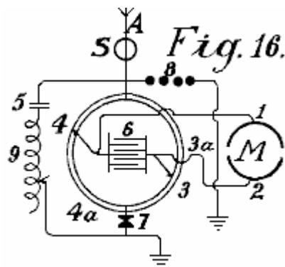
Fig.16 is an arrangement with coupling by capacitor.
