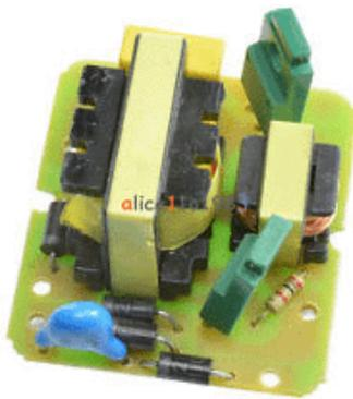
**12V to 220V Step UP Power Module 35W DC-AC Boost Inverter Module Dual Channel**
