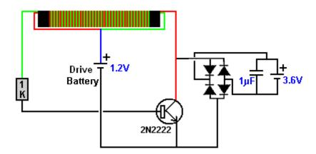
Without the charging battery connected, this circuit gives 28 volts on the capacitor and the battery charging is good, giving load testing results of 4.18, 4.16, 4.15, 4.13, 4.11, 4.10, 4.08, 4.08, 4.06, 4.05, 4.04, 4.03, 4.02, 4.00, 3.99, 3.98, 3.97, 3.96, 3.95, 3.95, 3.94, 3.94, 3.93, 3.93, and 3.93 volts after powering the load for 24 hours. This seems to be a very satisfactory result for such a minor alteration.
