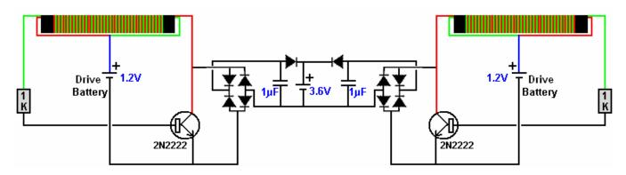
There is no need to restrict the battery on charge to a nominal 3.6 volts in any of these circuits as a single 1.2 volt drive battery can easily charge a 4.8 volt battery or larger. The value of the capacitor has a considerable effect and I suggest a one microfarad capacitor is a good choice. It has been argued that the two additional diodes on each side of the battery being charged are not necessary, although I have shown them to isolate the two circuits from each other.
