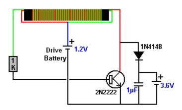
With the battery on charge removed, the voltage on the capacitor reaches 22 volts. Charging the same batteries with this circuit reached 4.14 volts and produced load results of 4.09, 4.05, 4.01, 3.98, 3.96,
