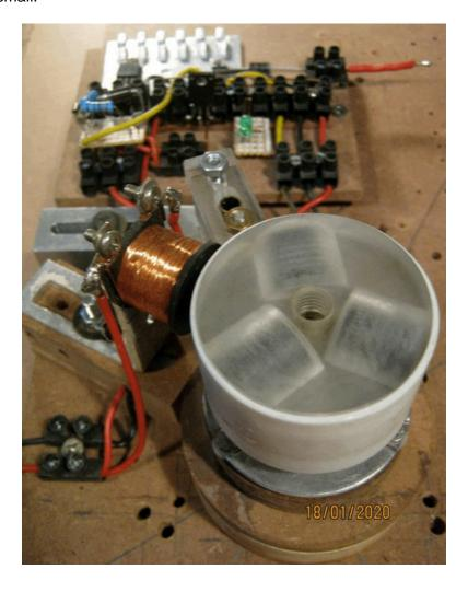
The sensor is positioned about 1.5 mm away from the rotor and the coil is on a solid metal core, which,
